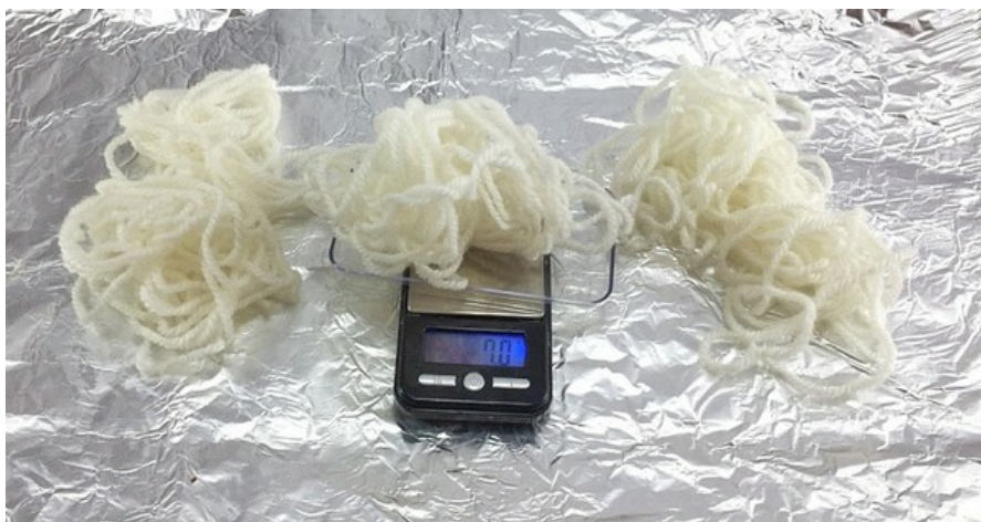
Figure 14. Weigh each piece of wool to find out how much grease the wool has taken up.
