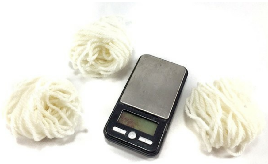
Figure 8. Each of the wool pieces should weigh approximately 5 g. Note: The wool yarn provided in the kit is much thinner than the wool yarn shown in this, and the following pictures.
