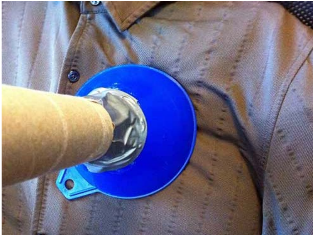
Figure 3. To listen to another student's heartbeat, have the listener place the funnel flat on the chest of the other student, on the left side roughly where the heart is. The listener should place his or her ear at the hole on the end of the tube, on the other end of the stethoscope.
