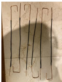
Figure 6: Copper wire bent for the electrodes. Photos taken by Brindha Srivatsav
