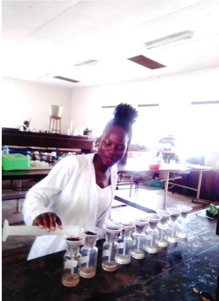
Figure 3. 11: Conducting a water retention test
