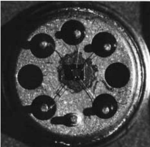
This detailed integrated circuit was too complex for raw lighting. Shadows and highlights are quite confusing, and the broken lead wire is difficult to see.
