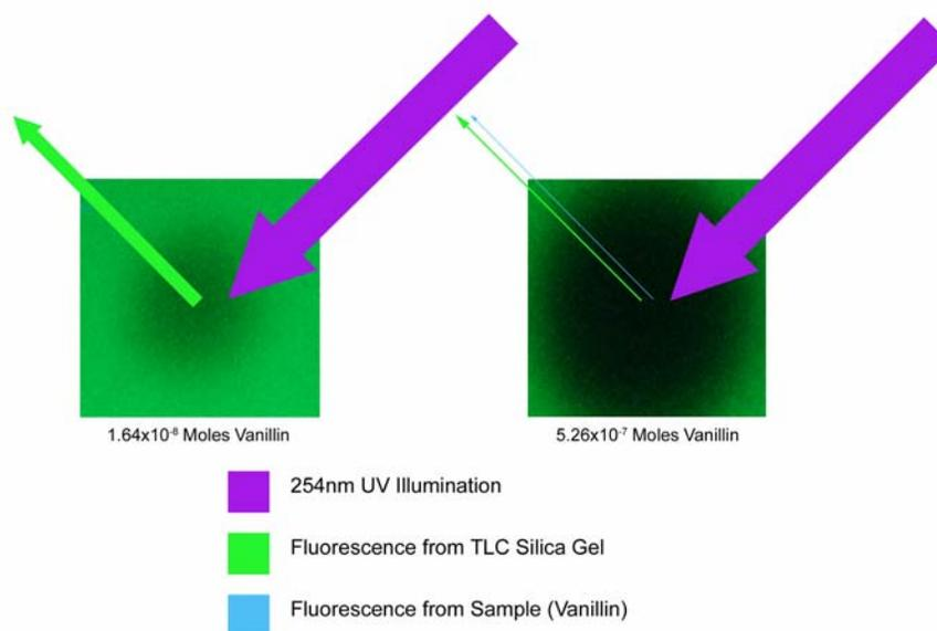
The lower the concentration of the sample on a TLC plate, the more 254 nm UV light that can go between molecules of the sample to reach the green fluorescing compound in the silica gel on the plate. As the concentration of the sample increases, less and less UV light reaches the silica gel and the spot becomes darker (unless it is an extremely bright fluorescent compound in its own right).
